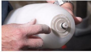
8. Sand flexible inner down so anchor is almost 100% exposed
