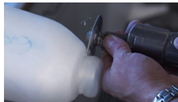
6. Cut tooling free with cast saw, knife or utility knife.
