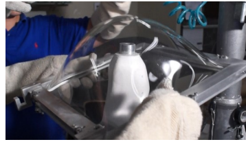
2. Pull preferred flexible plastic over socket and installed fabrication dummy using a vacuum system.
