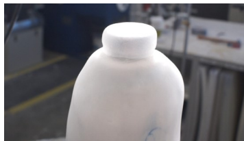
5. Let plastic cool before cutting fabrication dummy free.
