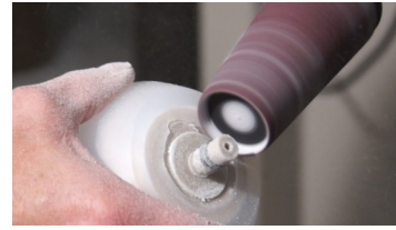
8. Sand flexible inner down so anchor is almost 100% exposed
