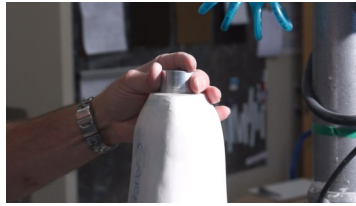
2. Pull preferred flexible plastic over socket and installed fabrication dummy using a vacuum system.
