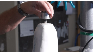
1. Put CD103FD fabrication dummy over anchor.
