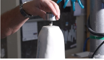
1. Put CD103FD fabrication dummy over anchor.
