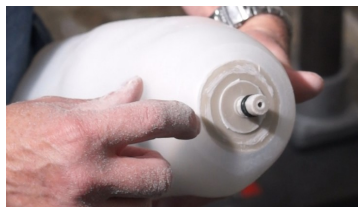
8. Sand flexible inner down so anchor is almost 100% exposed
