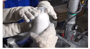
3. Pressing in around fabrication dummy will help remove any air pockets.
