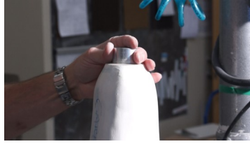
2. Pull preferred flexible plastic over socket and installed fabrication dummy using a vacuum system.
